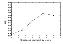
Fig. 1. SiO<sub>2</sub> content versus ultrasonic treatment time with +106 micrometer size fraction
